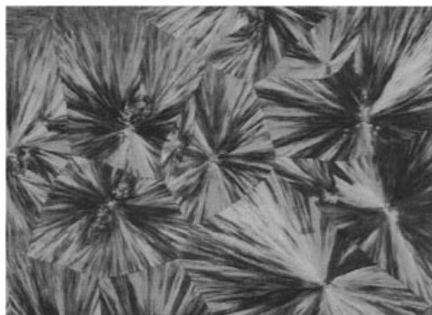
Figure 3. Optical micrograph obtained from a 0.3 g/g PEO/Urea, namely close to the stoichiometric composition.
